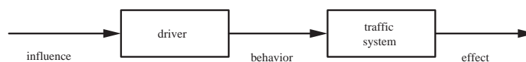
Figure 6.3: Model for the influence of traffic measures on the traffic system, after Van Altna and Veling (2000). Notice that this model fits within the model of internal and external influences (figure 6.1).
